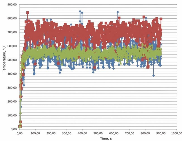
Fig. 4. Temperature readings of sensors along the perimeter of the fire test chamber walls at a height of 5.5 m (sensor layout according to the scheme in Fig. 2)
