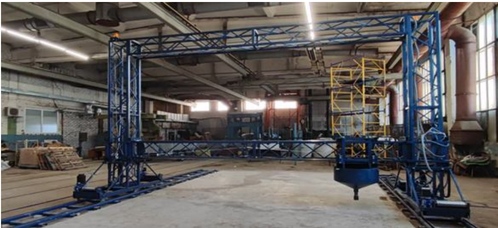
Fig. 2. Research 3D printer ("PSEIITC") of the Ukrainian State University of Science and technologies
