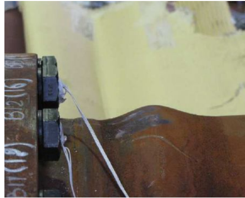
Fig. 12. Zone of local deformation of the pipe wall, experimental data [9]
