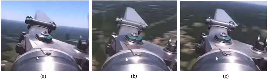
Fig. 1. Instantaneous camera photos of helicopter blade transverse movement: (a) lower position; (b) middle position; (c) upper position
