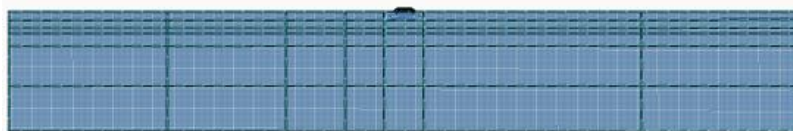
Fig. 1. Finite element model of the ballast prism and multilayer soil foundation
