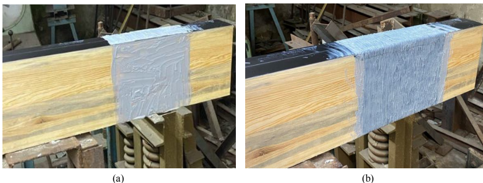
Fig. 9. Application of Sikadur-330 adhesive: (a) – applying Sikadur-330 adhesive to the model base; (b) – rolling in Sika Wrap - 230 C/45 fabric into Sikadur-330 adhesive on the model surface
