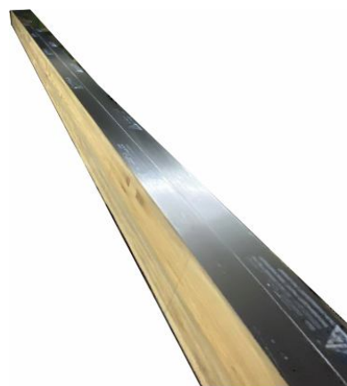
Fig. 8 Composite strips Sika CarboDur S-512 bonded to the glued laminated timber beam
