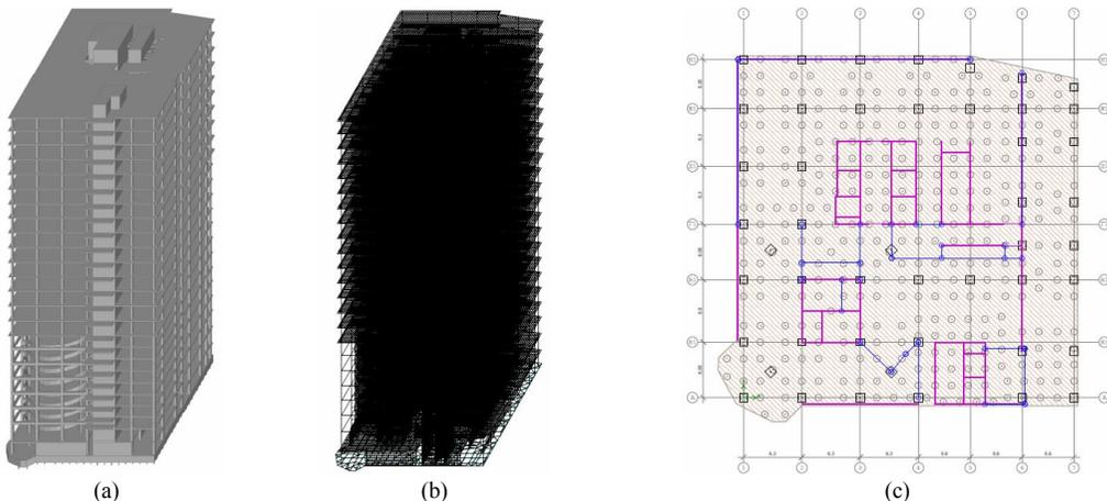
Fig. 6. (a) 3D scheme; (b) design scheme in SCAD; (c) basement floor plan, formwork of the monolithic raft foundation and pile field
