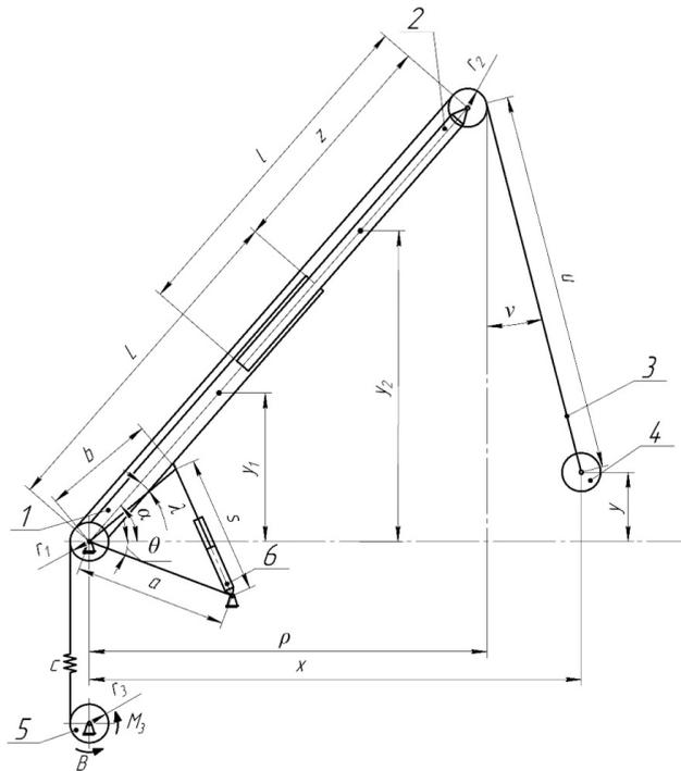
Fig. 1. Dynamic model of the crane jib system with joint operation of the mechanisms for changing the outreach and lifting the load at a steady-state crane rotation
