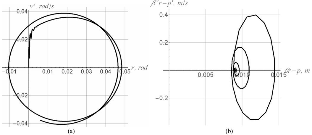
Fig. 7. The phase portraits of oscillations of a load on a flexible suspension (a) and a traction rope (b) of the lifting mechanism
