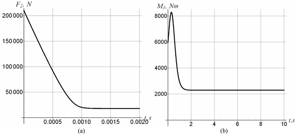
Fig. 11. The graph of the driving force of the hydraulic cylinder of the boom extension section (a) and the driving torque on the drum of the lifting mechanism (b)
