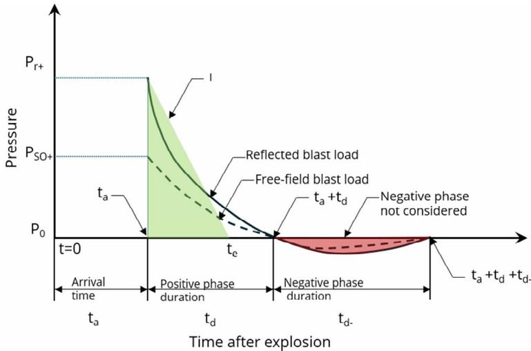
Fig. 5. Simplified graph of pressure change during an explosion
