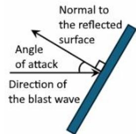
Fig. 2. Reflected angle of incidence of the blast wave
