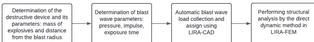
Fig. 8. Algorithm for analysis of structures under the influence of an explosive blast wave by the direct dynamic method
