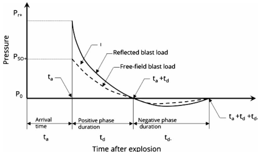
Fig. 1. Pressure change in a blast wave with time at a fixed point
