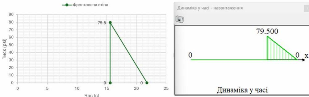
Fig. 6. Pressure versus time plot for the wall facing the explosion
