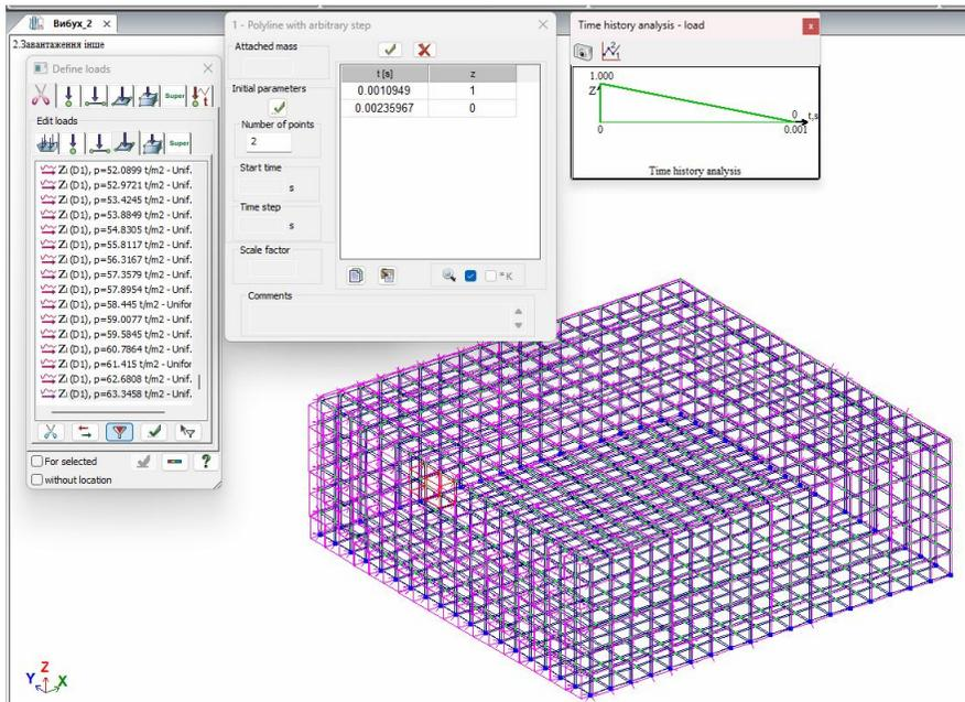
Fig. 7. Automatic collection of loads on elements with a given dynamic impact rule for analysis by the direct dynamic method
