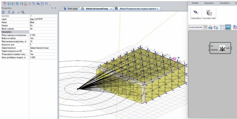
Fig. 4. Creation of a model of loads on a plate structure under the action of a blast wave in LIRA-FEM
