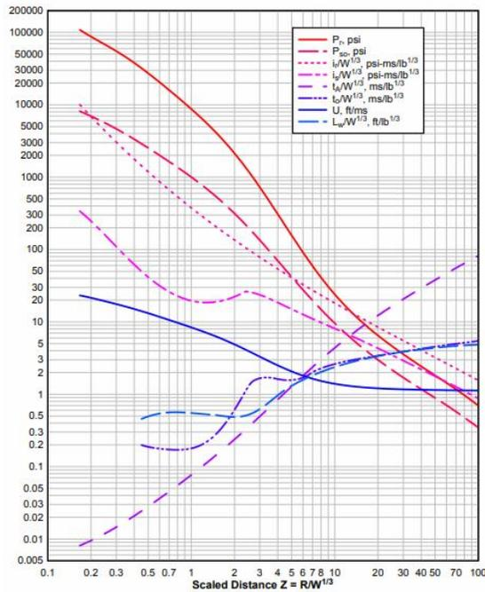
Fig. 3. Parameters of the positive phase of the blast wave for surface explosions
