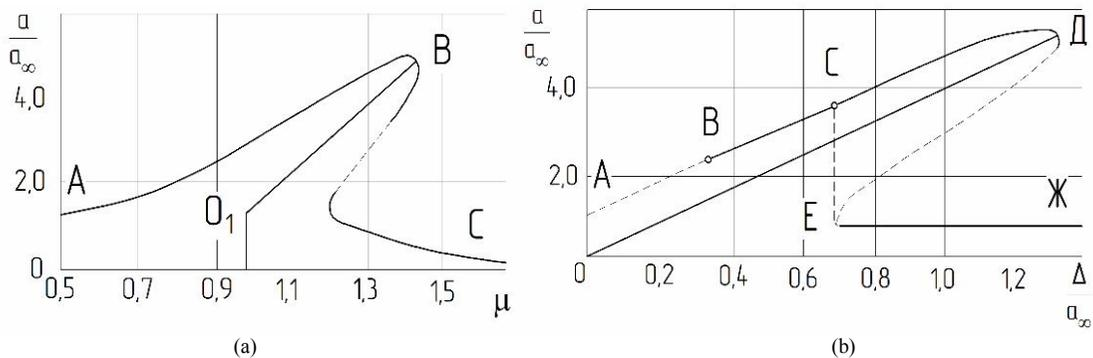
Fig. 4. Skeletal and amplitude curves of the vibration installation: (a) at  $\Delta/a_0 = 1,36$ , (b) at  $\mu = 1,5$
