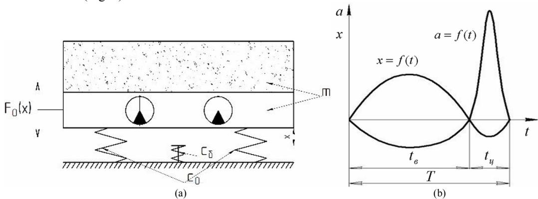
Fig. 3. Vibration shock installation: (a) - design model; (b) - change of displacement and acceleration during the period of oscillation
