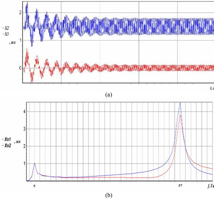
Fig. 2. Amplitudes of mass oscillations  $m_1$  and  $m_2$  and graph of the amplitude and frequency response of the vibration installation
