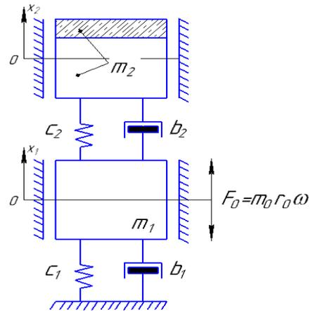
Fig. 1. Design diagram of a two-seater vibration unit
